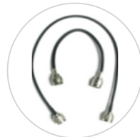
Feeder connects external duplexer and repeater
